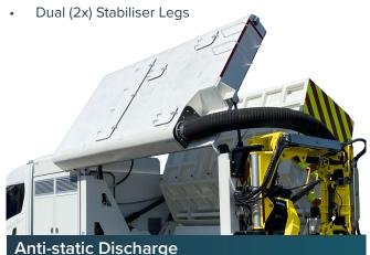
14m retractable rear-mounted earthing hose reel
